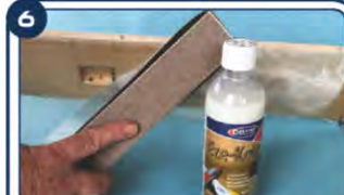
6 Excess fabric is effortlessly trimmed away using a Perma-Grit sanding block or 320 grit paper.
