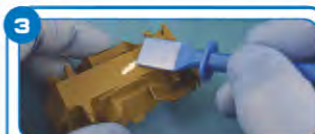
Use the spatula to spread the putty. Once dry, polish carefully with a fine grade sanding stick.
