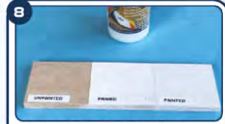
8 Having sanded the wing, we tested Halfords White primer, and our chosen paint, Halfords Spray Ford Diamond White. Eze-Kote has good compatibility with most white car primer paints. If you're in doubt always check by testing the primer and paint top coat before committing to the model.
