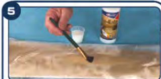
5 Eze-Kote is then brushed through the glass fibre fabric. Note that any unused Eze-Kote can be returned to its container.
