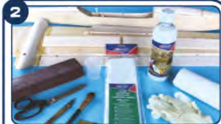
2 Eze-Kote with the 0.6 oz Super Lightweight Glassfibre laminating fabric (BD11), gloves, brushes, and scissors that you would need to undertake the Eze-Kote process.
