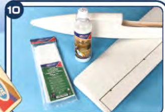
10 A second coat of Eze-Kote is applied after the glass cloth has been trimmed. After sanding and further filling if required, the model is ready for painting.
