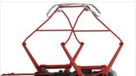
Elegant pantograph type SBS 54/10 with invisible fastening
