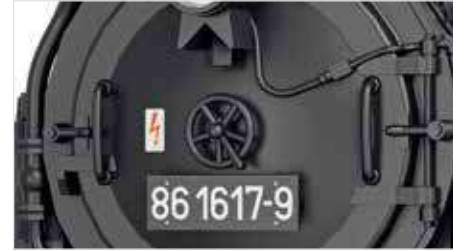
Elaborate smoke chamber door
