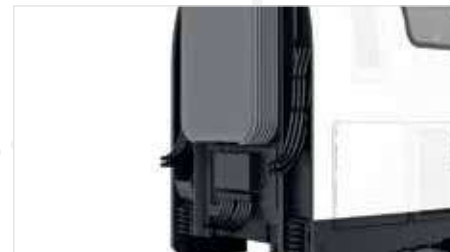
Reproduction of the cables between the coaches
