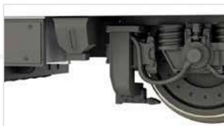
Reinforced design of the sand downpipes
