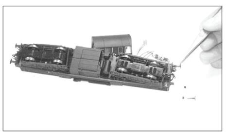
1. Gently remove the driver's cabin as described on page 1. Remove the 'rings' that attach the buffers to the buffer beam in one of the ends of the loco and the buffers can be removed.
