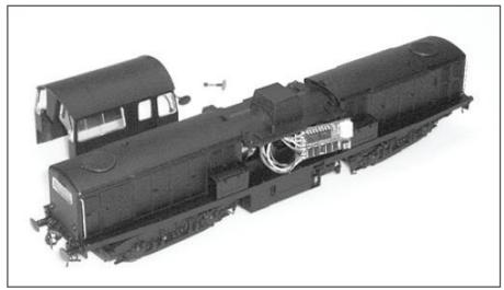
Your Class 17 will operate in DCC mode with any compatible 8-pin DCC decoder. It is also possible to install DCC sound using a suitable decoder and speaker but as internal space is limited we recommend consulting a professional DCC sound specialist to advise on the relevant components.
