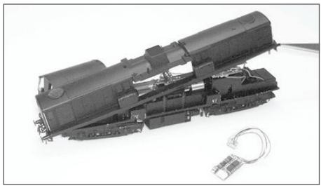
2. Lift the bodyshell and you will gain access to the motor and printed circuit. Remove the dummy plug.
