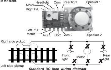
The 'X' marks indicate where to disconnect (isolate).
