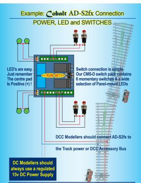
Important: AD-S2fx has a high power CDU on each of its outputs. Allowing the lower face of the PCB to contact conductive areas, metal tools etc. will cause serious damage to on-board electronics.
