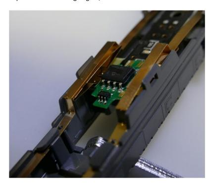
So it should slide in all the way without heavy resistance, for those who want to know the decoder does not reverse the polarity for the front and rear lights – it has separate outputs hence the 4 contacts on one side.
