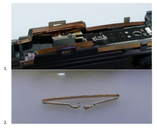
As you can see there are two sets of contacts, for reference to sprung brass is all one thing as seen in picture 2
