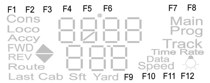
FWD / REV and SPEED icons display the loco speed and direction of travel The LAMP icon (F0) illuminates when the loco lights are activated
