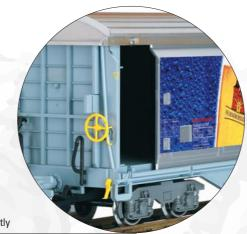
The sliding door can be unlocked by pulling slightly
