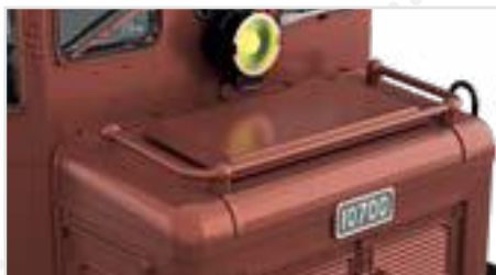
Free-standing handrails and separately-applied cover on the front end
