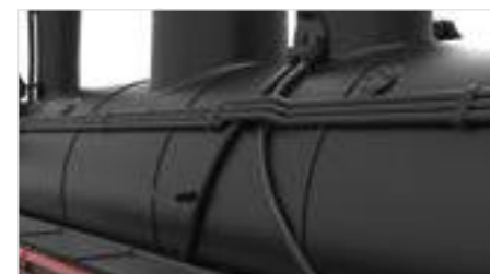
Separately attached boiler pipes
