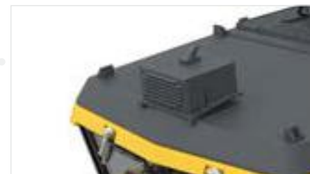
Separately attached signal horn box
