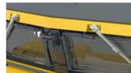
Plug-in windshield wipers and sockets
