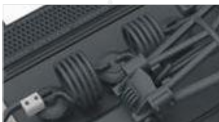
Interference current filter made from finest metal wire
