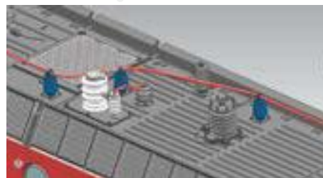
New main switch and primary voltage converter
