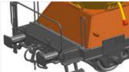
Detailed shunting platform with perforated grid
