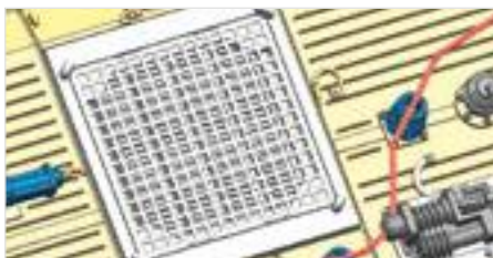
Brake tower grid made from fine etching sheet
