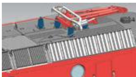
Separately applied cable to the current collectors
