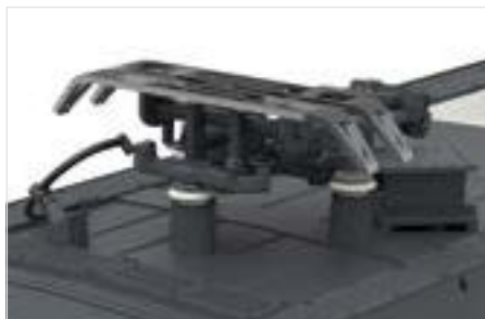
New current pantograph design with invisible mounting
