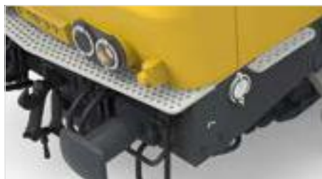
Running boards made from perforated metal
