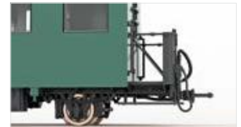
Platform area features almost-invisible coupling mounting
