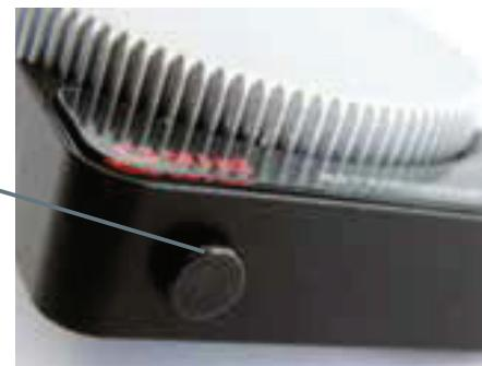
**The status-LED** displays the current state of your system. If the LED is green you can control and steer as you like. If the LED is red the PIKO SmartBox® either detected a short circuit or you triggered an emergency-stop.
