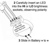
As soon as you fit the battery the LED should light because you are moving the module - if the LED does not light try fitting the LED the other way. Place the module on a completely still surface & just over 4 minutes after the last motion the LED should switch off.
