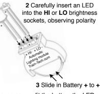
As soon as you fit the battery the LED should light because you are moving the module - if the LED does not light try fitting the LED the other way. Place the module on a completely still surface & just over 4 minutes after the last motion the LED should switch off.
