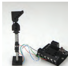
Signal with a feather connected to an SC2
