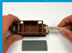
1 Remove roof and drill two small holes for LED
