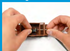
2 Fit module inside, plug in LED & battery
