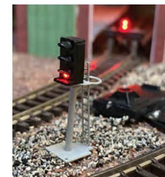
Gaugemaster N gauge signal GM275 controlled automatically by an SC100
