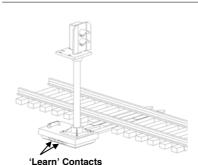
Touch together contacts under base to program Signal address
