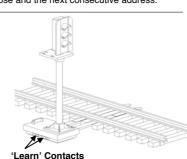
Touch together contacts under base to program Signal address
