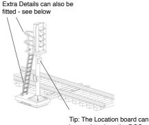
be used to show the DCC address of your signal to make it easier to identify you can cut out and glue the address from the table printed below
