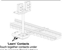
Touch together contacts under base to program Signal address
