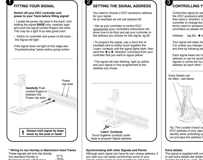
Bachmann tracks which have slots for a power clip. If you do not have this type of track or want to position your signal in a different place you can carefully cut off contact fingers where shown and connect wires from the 2 contacts
