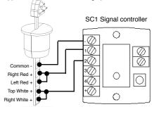
Wiring to SC1 DCC - White & single red or white This wiring is DCC control between single top white or single left red with a constantly lit right white. Follow instructions supplied with SC1 for setting up.
