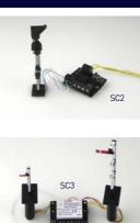
SC2 3 or 4 aspect or 2 aspect+route signal control Controls one 3 aspect or one 4 aspect or one 2 aspect + route signal Compatible with Train-Tech SK4 SK5 SK6 and most other manufacturer's LED signals SC3 Dual Dapol 00/N Sempahore signal controller Controls one or two standard OO or N Dapol motorised semaphore signals by DCC. Signals connect direct to
