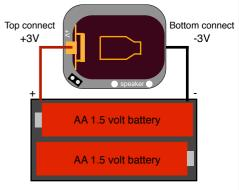
WARNING: Correct polarity & 3 volts MAXIMUM!
