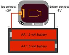
WARNING: Correct polarity & 3 volts MAXIMUM!
