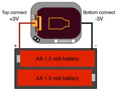
WARNING: Correct polarity & 3 volts MAXIMUM!
