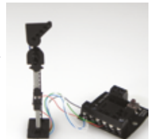
Signal with a feather connected to an TTSC2
