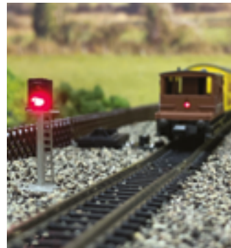
Gaugemaster N gauge signal GM270 controlled automatically by a TTSC100
