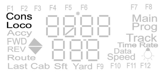
The MAIN / PROG / TRACK and DATA icons are displayed in programming and (READ) modes, the SFT (shift) icon is used in function selection and when selecting in READ mode
