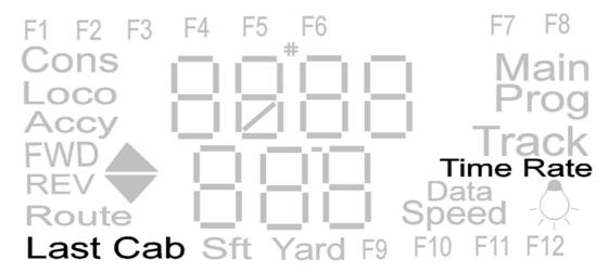
The LOCO and CONS icons are displayed when operating and programming locomotives and consists (DBL HEAD)
