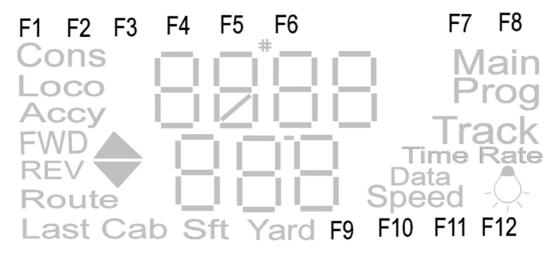
FWD / REV and SPEED icons display the loco speed and direction of travel The LAMP icon (F0) illuminates when the loco lights are activated
