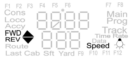
The LAST CAB icon is used in the system setting and the TIME RATE icon is displayed when operating the (fast clock) time mode
