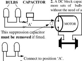
**2.** A DC block capacitor must be used in each feed. However more sets of bulbs can be added at points marked 'A' without the need of additional capacitors.
