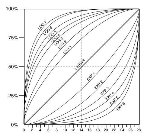
The speed curves can be used in 14, 28 and 128 speed step modes.
