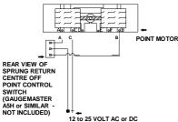
12 to 25 VOLT AC or DC (+VE & -VE OUTPUT TERMINALS OF CAPACITOR DISCHARGE UNIT IF USED)
